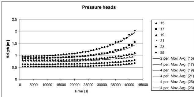
Fig. 9. Evolution of pressure head for different piezometer positions for dams with permanent storage
