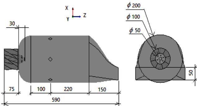
Fig. 2 Dimensions of combustor flow domain. All dimensions are in mm.
