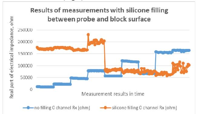
Fig.7 EIS measurements during the drying process of the reference block and block with silicone filling between the probe and the measurement surface
