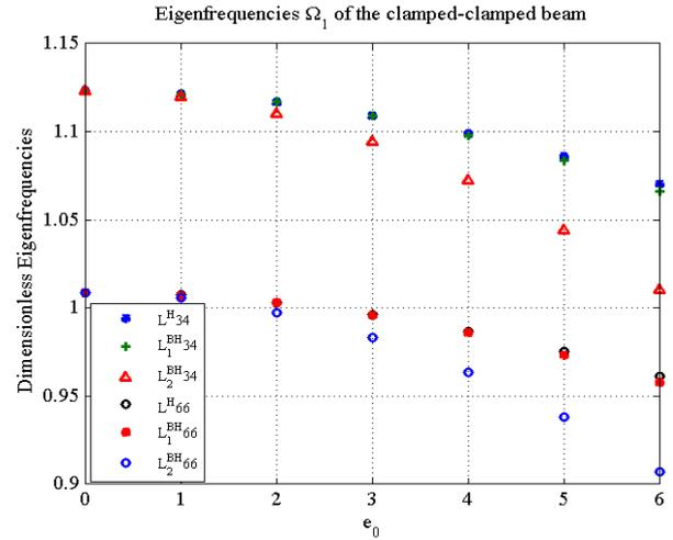
Figure 5 The  $\Omega_1$  eigenfrequency of the clamped-clamped beam Vs nonlocal parameter  $e_0$  for the case of  $L^H$ ,  $L_1^{BH}$ ,  $L_2^{BH}$
