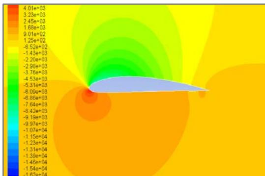
Fig. 4 airfoil without cavity: pressure distribution
