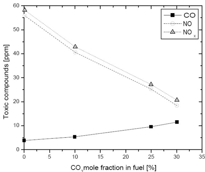
Fig. 11 Emission of NO, NO<sub>x</sub> and CO vs. CO<sub>2</sub> content in Combustion mixture
