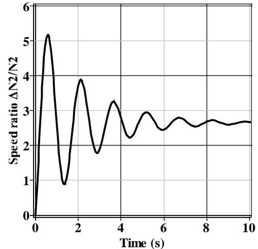
Fig. 2 step response of the HPC rotational speed to the fuel flow rate input
