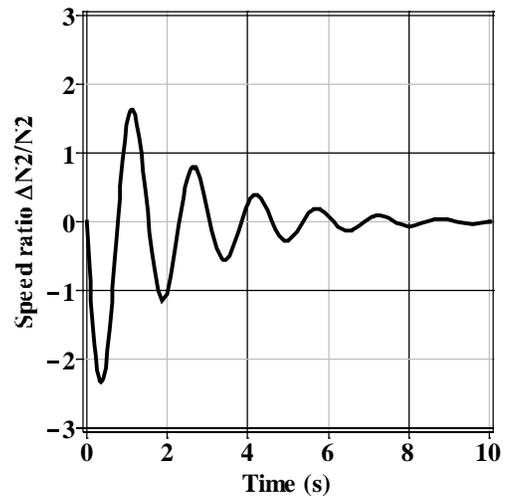
Fig. 7 impulse response of the HPC rotational speed to the nozzle area input
