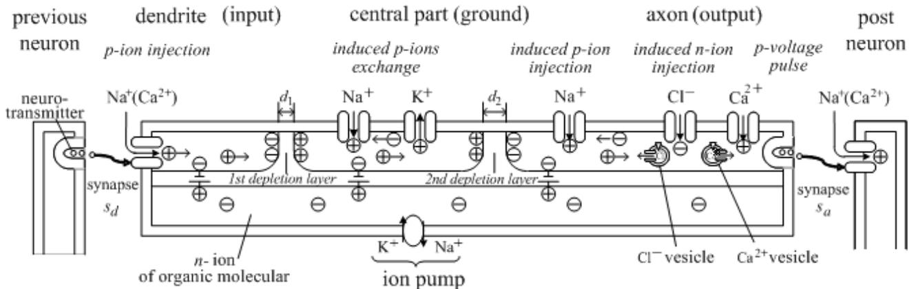
Fig. 3 Electro-physical modeling of an operating neuron. All branches of the dendrite and the axon of a neuron are gathered into each one port. Ion channels of the same kind are gathered in one in an area.
