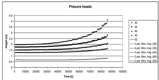
Fig. 14. Evolution of pressure heads for different piezometer positions for dams with permanent storage
