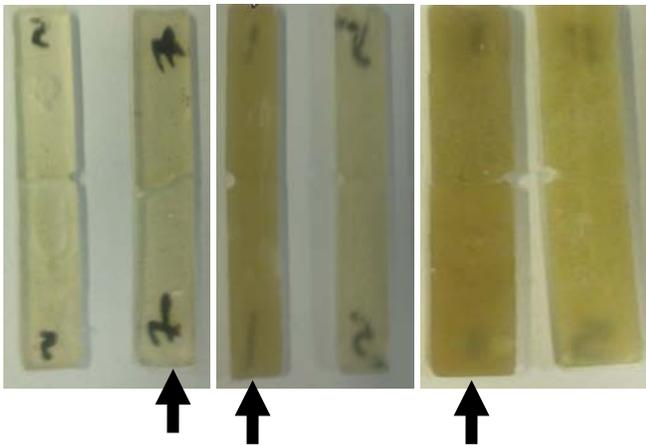
Figure 6 Appearance of Izod bars of PLA 2003D/clay composites. Arrows indicate samples prepared by LME plus LMM.
