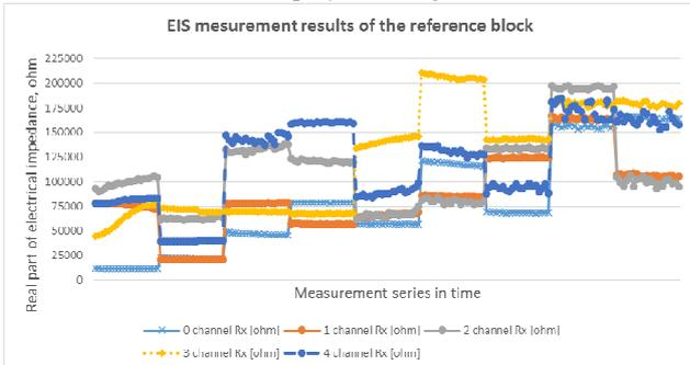
Fig.5 EIS measurements during the drying process of the reference block
