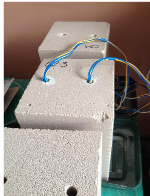
Fig.4. Autoclaved aerated concrete blocks with liquid silicone filling in bores and bores with no filling
