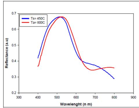
Fig.5: Reflectance spectra of CuFeO<sub>2</sub>/quartz thin film deposited at T<sub>s</sub>=450 °C and annealed at T<sub>a</sub>=800 °C.
