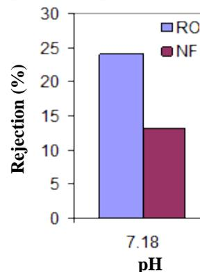
Fig 6. Effect of pH on removing sodium ions using RO and NF membranes
