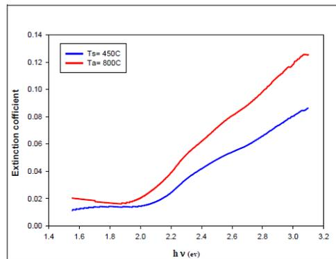
Fig.7 Extinction coefficient of CuFeO<sub>2</sub>/quartz thin film deposited at T<sub>s</sub>=450°C and annealed at T<sub>a</sub>=800°C
