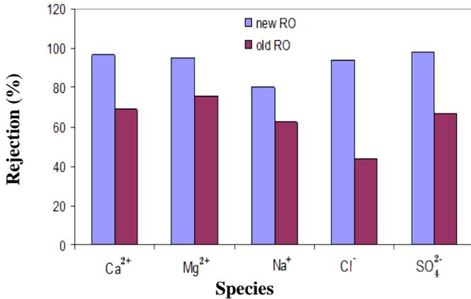
Fig 7. Comparison of the performance of RO membranes during three years operation
