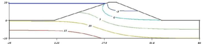
Fig. 12. Linear water level rise from 3.3 to 9.50 m
