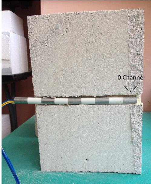
Fig.1. Cross section of autoclaved aerated concrete block used for the experiment with measurement probe
