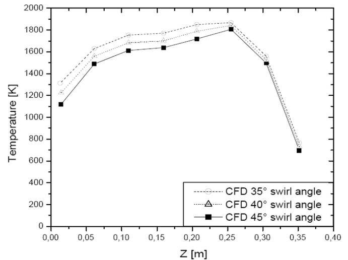
Fig. 5 Axial temperature for the can-combustor with different swirler angles
