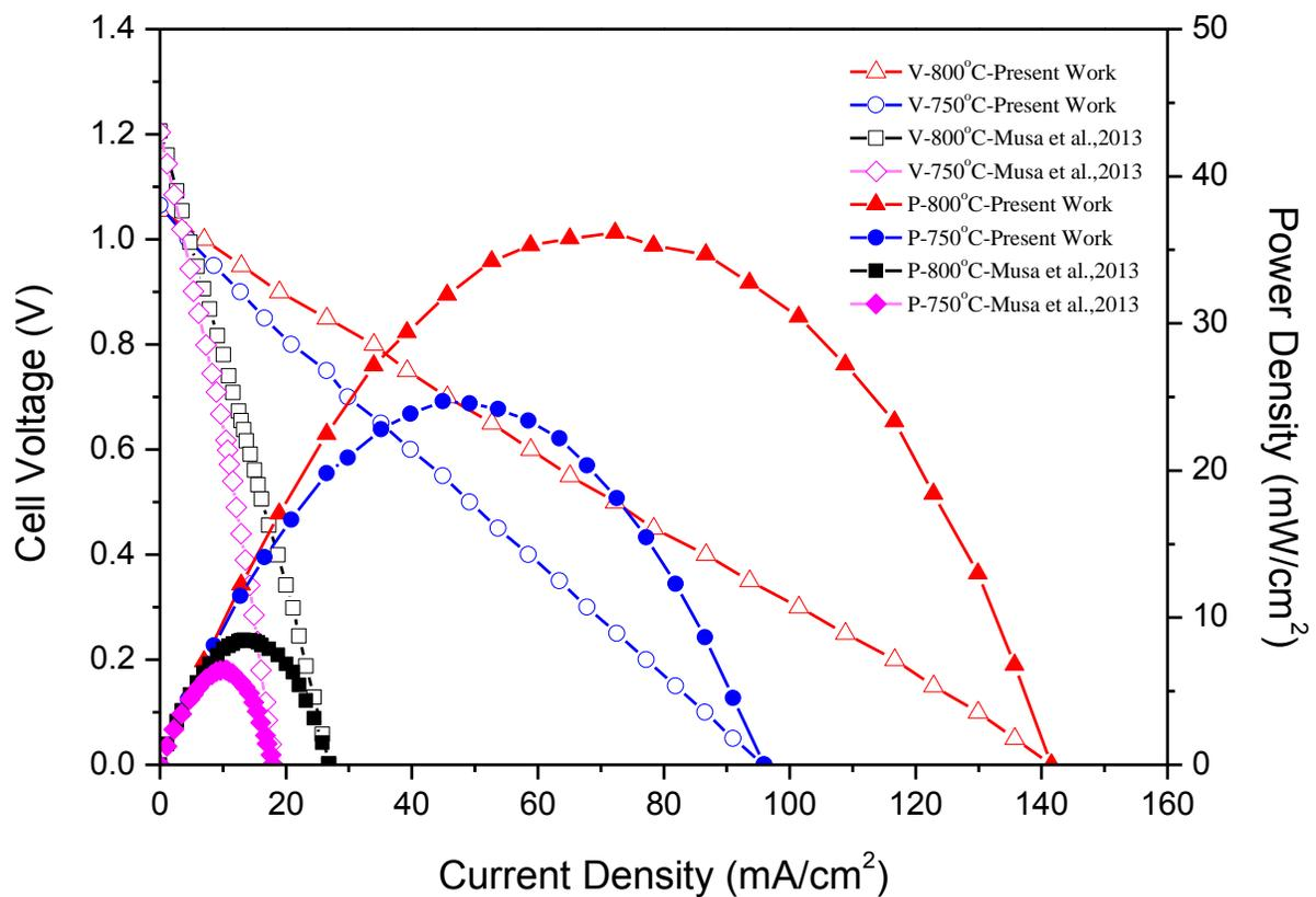
Fig 5. I-V-P Steady state results of Co-CeO<sub>2</sub>/ScSZ/LSM cells with anodes made by SP and conventional methods.
