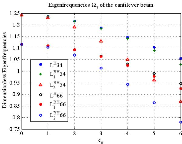
Figure 4. The  $\Omega_3$  eigenfrequency of cantilever beam Vs nonlocal parameter  $e_0$  for the case of  $L^H$ ,  $L_1^{BH}$ ,  $L_2^{BH}$ . [The number (34 or 66) after the  $L$  and before the index is the thickness of nanotube (0.34nm or 0.066nm respectively)]
