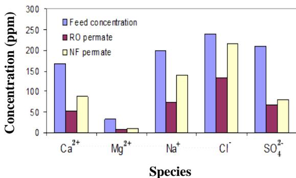
Fig 4. Comparison of the performance of old RO and old NF membranes
