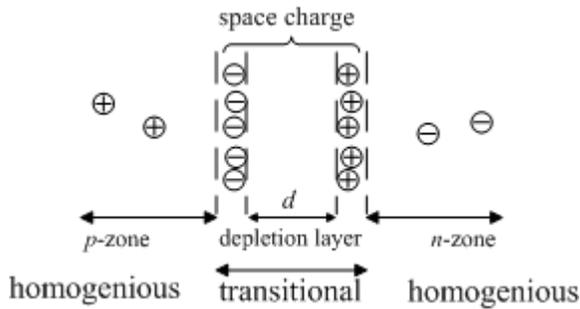
Fig. 1 Formation of zones and a depletion layer at a boundary.
