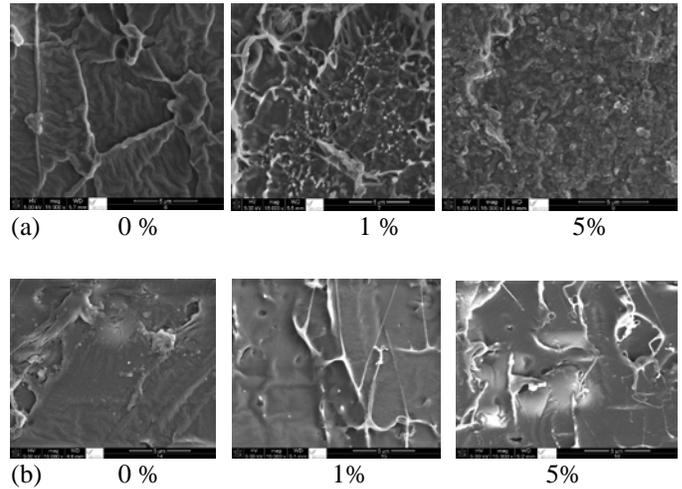
Figure 8 SEM micrographs of Izod samples of PLA 6752D with various weight percents of clay. (a) processed by LME followed by LMM. (b) processed by LMM only.
