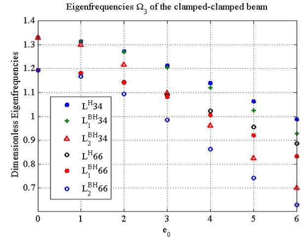
Figure 6. The  $\Omega_3$  eigenfrequency of the clamped-clamped beam Vs nonlocal parameter  $e_0$  for the case of  $L^H$ ,  $L_1^{BH}$ ,  $L_2^{BH}$
