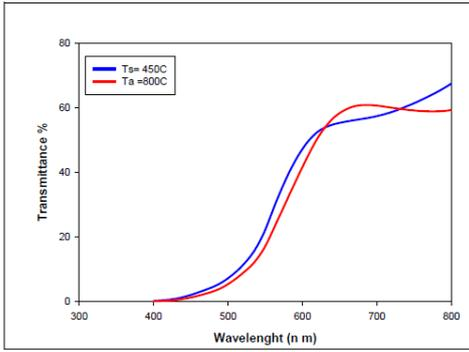
Fig.2 : Transmittance spectra of CuFeO<sub>2</sub>/quartz thin films deposited at T<sub>s</sub>= 450 °C and annealed at T<sub>a</sub>=800° C.
