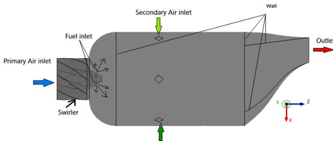
Fig. 1 Solid model of combustor flow domain.
