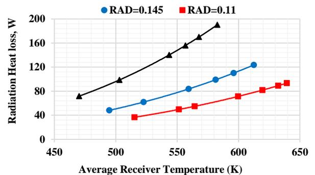
Figure 4: Effect of average receiver temperature on radiation heat loss, receiver emissivity=1 and  $I=1000 \text{ W/m}^2$
