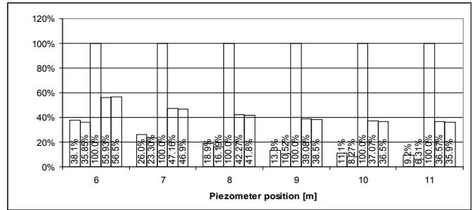
Fig. 5. Comparison of the piezometric surface in different scenario compared with steady seepage
