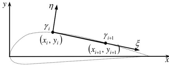
Fig. 12 vortex panel coordinate system
