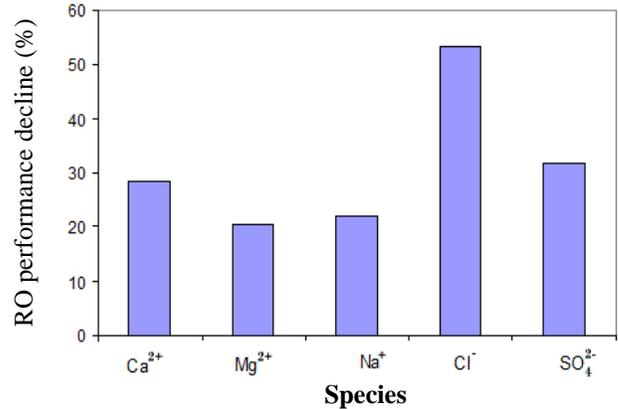
Fig 9. Percentage decline of the performance of RO during three years operation
