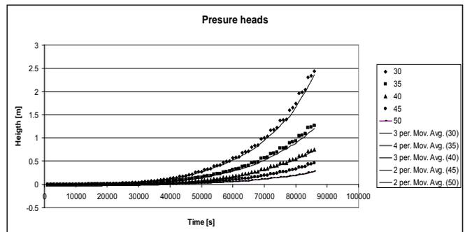
Fig. 13. Evolution of pressure for different piezometer positions for dams with non permanent storage
