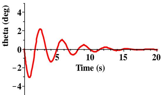
Fig. 11 pitch angle impulse response.
