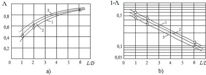
Fig.1. A relative level of magnetization of filter-matrix samples (a), and the shortage of this level (b) varying with their relative dimension by data in [6] (points), 1- $H=30$  (kA/m) ( $\mu=8.5$ ), 2- $H=60$  (kA/m) ( $\mu=7.4$ ), 3- $H=80$  (kA/m) ( $\mu=6.9$ ). The lines are the calculation according to (6) and (8).
