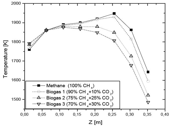
Fig. 8 Distribution of temperature along the center line of combustor.
