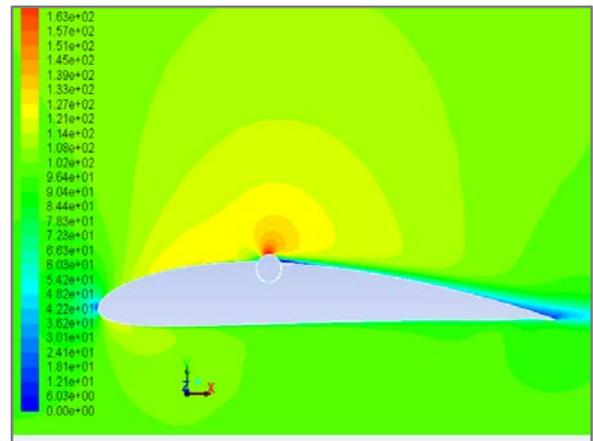
Fig. 7 airfoil with filled cavity: velocity distribution
