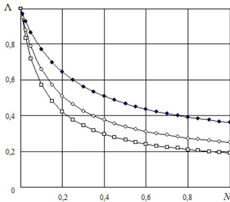
Fig. 3. Relative level of magnetic body magnetizing depending on its demagnetizing factor 1 –  $\mu=5$ ; 2 –  $\mu=7.5$ ; 3 –  $\mu=10$ .
