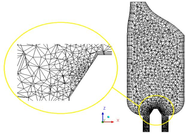
Fig. 4 Mech geometry of gas turbine can combustor (midaxial vertical plane).
