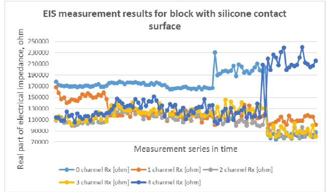
Fig.6 EIS measurements during the drying process of the block with silicone filling between the measurement probe and the surface of the aerated concrete block
