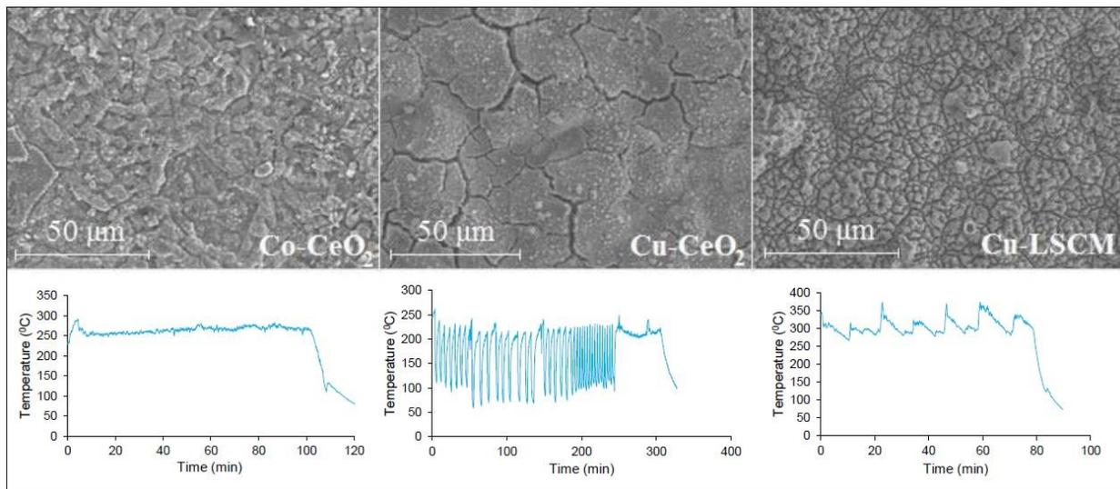
Fig 3. Anodic electrodes prepared by sp with corresponding substrate temperatures variation.
