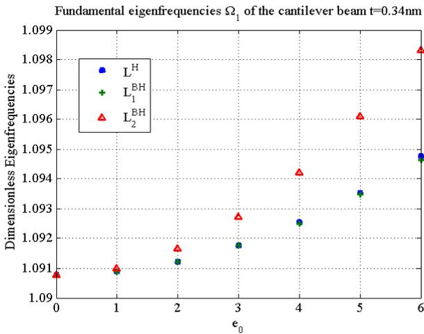
Figure 3. The  $\Omega_1$  eigenfrequency of cantilever beam Vs nonlocal parameter  $e_0$  for the case of  $L^H$ ,  $L_1^{BH}$ ,  $L_2^{BH}$ .
