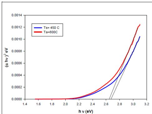
Fig.4: Direct energy band gap of CuFeO<sub>2</sub>/quartz thin film deposited at T<sub>s</sub>=450C and annealed at T<sub>a</sub>= 800C.
