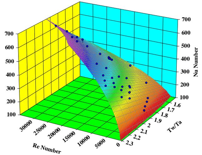
Figure 9: Variation of  $Nu$  number with receiver wall temperature ratio and  $Re$  number
