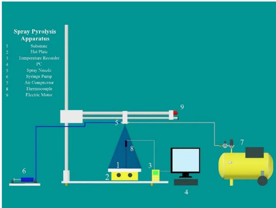
Fig. 1 Spray Pyrolysis apparatus
