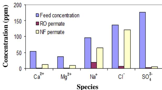
Fig 3. Comparison of the performance of new RO and new NF membranes
