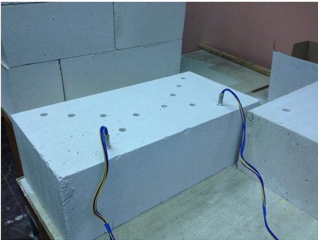
Fig.2. Autoclaved aerated concrete block with one pair of measurement probes
