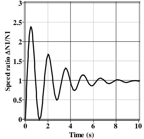
Fig. 1 step response of the LPC rotational speed to the fuel flow rate input
