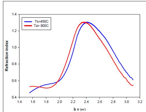
Fig.6:Refractive index of CuFeO<sub>2</sub>/quartz thin film deposited at T<sub>s</sub>=450°C and annealed at T<sub>a</sub>=800°C.
