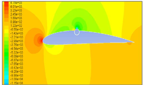
Fig. 5 airfoil with filled cavity: pressure distribution
