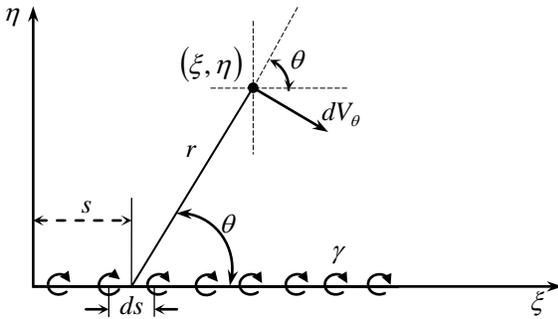
Fig. 13 edge view of a 2-D vortex panel
