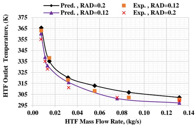
Figure 10: The effect of HTF mass flow rate on HTF outlet temperature for a conical receiver,  $I=1000 \text{ W/m}^2$
