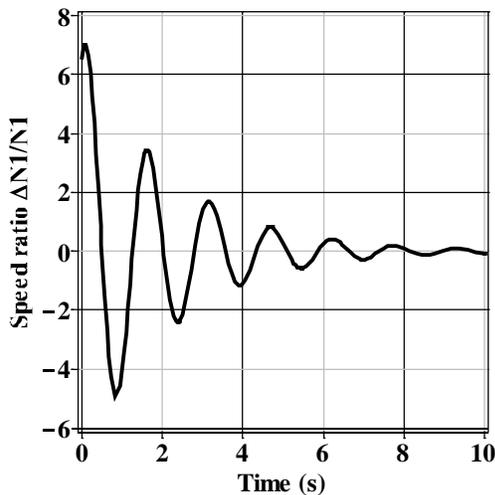
Fig. 5 impulse response of the LPC rotational speed to the fuel flow rate input
