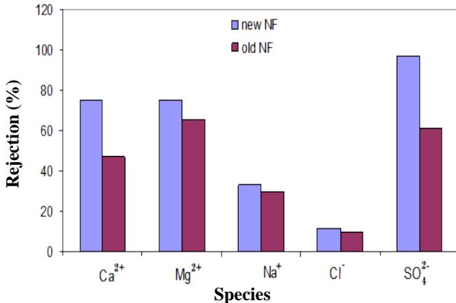
Fig 8. Comparison of the performance of NF membranes during three years operation
