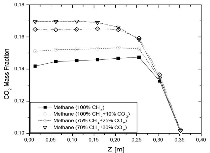
Fig. 10 Distribution of CO<sub>2</sub> mass fraction along the center line of combustor.
