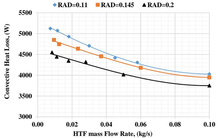
Figure 6: The effect of HTF mass flow rate on convection heat loss, receiver emissivity=1 and I=1000 W/m<sup>2</sup>
