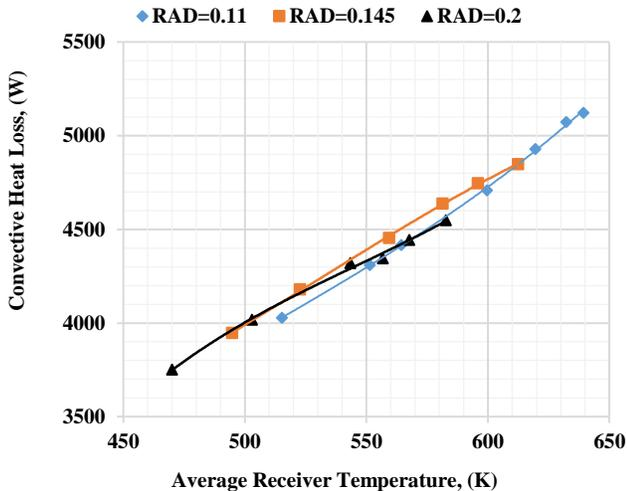
Figure 5: Effect of average receiver temperature on convection heat loss, receiver emissivity=1 and I=1000 W/m<sup>2</sup>
