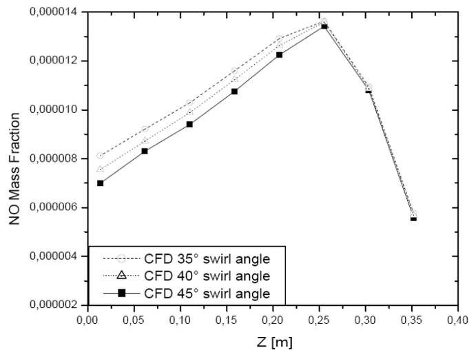
Fig. 6 Axial  $\text{NO}$  mass fraction for the can-combustor with different swirler angles
