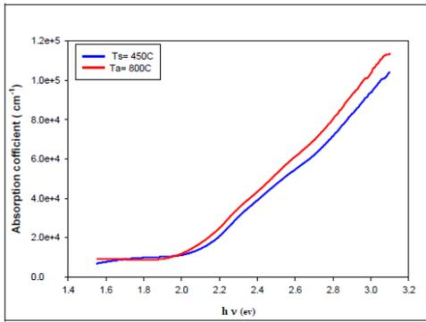
Fig.3 Absorption coefficient of CuFeO<sub>2</sub>/quartz thin films deposited at T<sub>s</sub>= 450 °C and annealed at T<sub>a</sub> = 800 °C.
