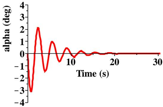
Fig. 9 angle of attack impulse response
