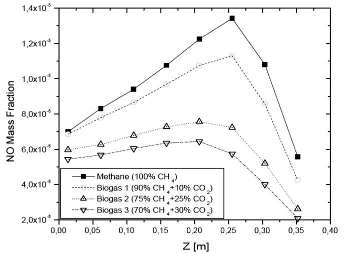
Fig. 9 Distribution of NO mass fraction along the center line of combustor.
