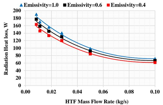
Figure 3: Effect of HTF mass flow rate on radiation heat loss for receiver with different wall emissivity for  $RAD=0.2$  and  $I=700 \text{ W/m}^2$
