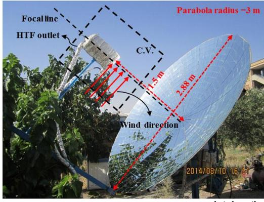
Figure 1: The photo of dish with cylindrical receiver
