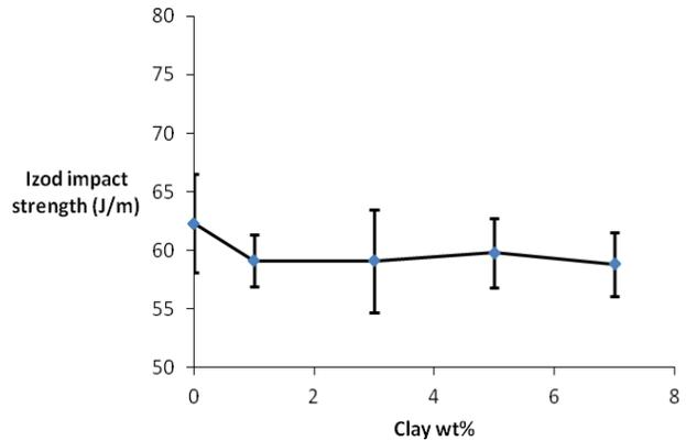
Figure 2 Tensile and impact strength of PLA6751D/clay composites.
