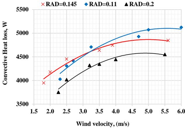
Figure 8: The effect of wind velocity parallel to concentrator plane on convection heat loss, HTF mass flow rate=0.09 kg/s,  $I=700$  W/m<sup>2</sup> and receiver emissivity is 1.
