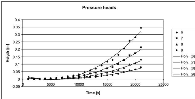
Fig. 3. Evolution of pressure head for different piezometer positions for dams with non permanent storage
