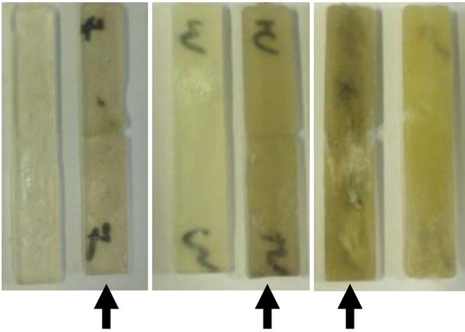
Figure 5 Appearance of Izod bars of PLA 6752D/clay composites. Arrows indicate samples prepared by LME plus LMM.
