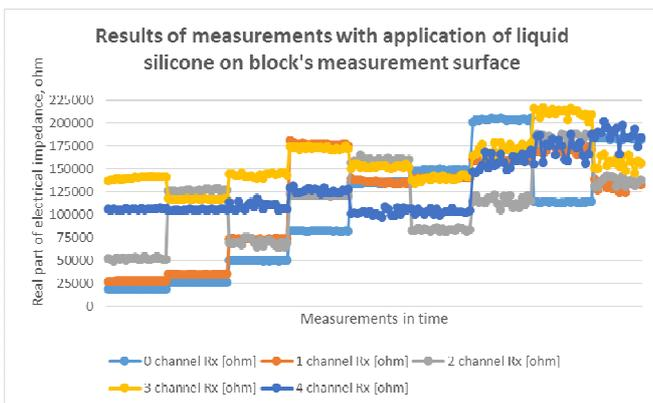
Fig.8 EIS measurements during the drying process of block with liquid silicone spray filling between the probe and the measurement surface
