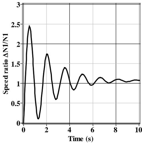
Fig. 3 step response of the LPC rotational speed to the nozzle area input
