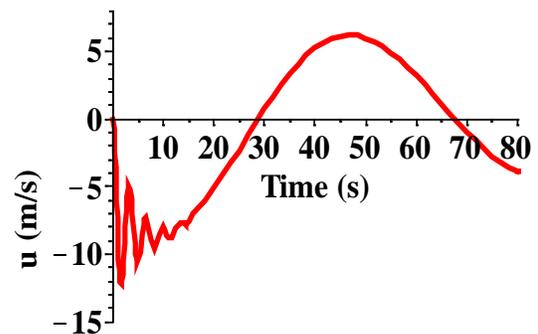
Fig. 8 aircraft velocity impulse response
