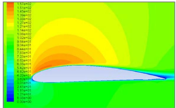
Fig. 6 airfoil without cavity: velocity distribution
