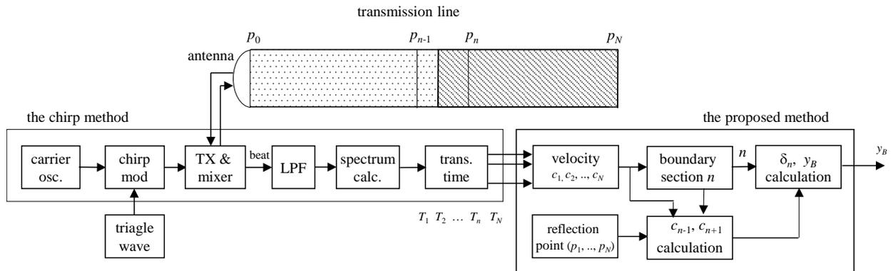
Fig. 2 System configuration of electrical measurement scheme.
