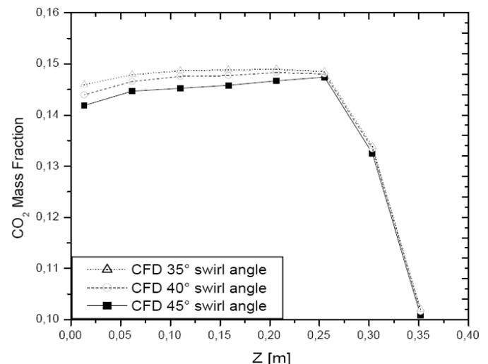
Fig.7 Axial  $\text{CO}_2$  mass fraction for the can-combustor with different swirler angles
