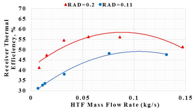
Figure 7: The effect of HTF mass flow rate on receiver thermal efficiency, receiver emissivity=1 and I=800 W/m<sup>2</sup>
