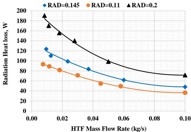
Figure 2: Effect of HTF mass flow rate on radiation heat loss for receiver with different aperture diameters, receiver emissivity=1 and  $I=700 \text{ W/m}^2$
