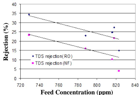
Fig 5. Percentage rejection of TDS versus feed concentration for RO and NF membranes
