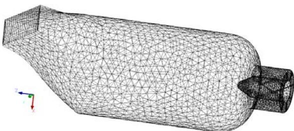
Fig. 3 Combustor computational mesh.
