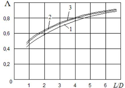
Fig. 4. Calculation data obtained according to (12), the data of relative magnetization level of filter-matrix samples in terms of their relative size, 1– $\mu=8.5$ , 2– $\mu=7.4$ , 3–  $\mu=6.9$ .
