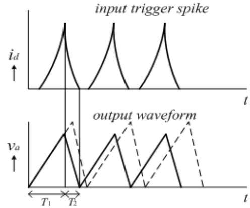
Fig. 6 Astable pulse generator by external injection. Dotted line is an original waveform. Solid line is the waveform synchronized to input trigger pulse.
