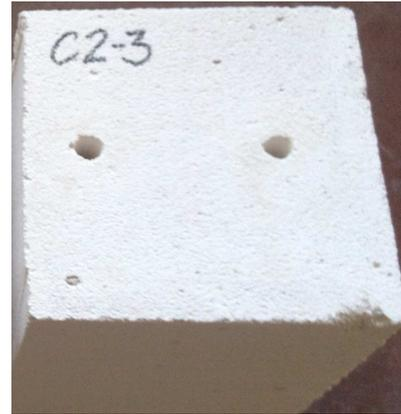
Fig.3. Autoclaved aerated concrete block used for the experiment
