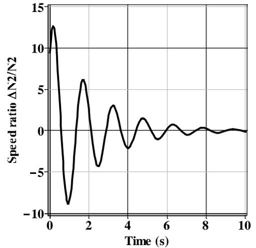
Fig. 6 impulse response of the HPC rotational speed to the fuel flow rate input
