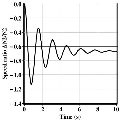
Fig. 4 step response of the HPC rotational speed to the nozzle area input
