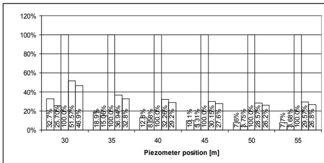
Fig. 15. Comparison of the piezometric surface in different scenario compared with steady seepage
