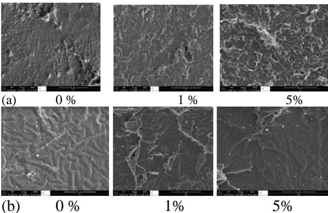
Figure 7 SEM micrographs of Izod samples of PLA 2003D with various weight percents of clay. (a) processed by LME followed by LMM. (b) processed by LMM only.
