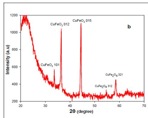
Fig.1: XRD pattern for CuFeO<sub>2</sub> thin films prepared using chemical spray pyrolysis (a: T<sub>s</sub> = 450°C (b: T<sub>a</sub> = 800 °C).
