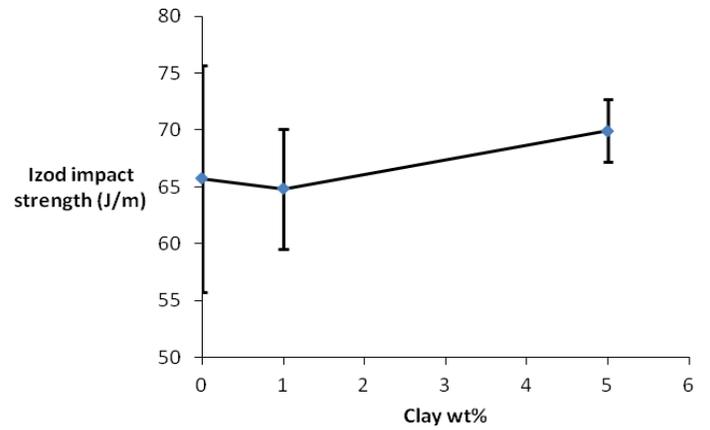
Figure 3 Tensile and impact strength of PLA (2003D)/ clay composites prepared by LMM only.
