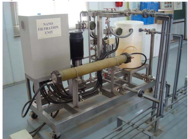
Fig 2. Systemic layout of nanofiltration unit
