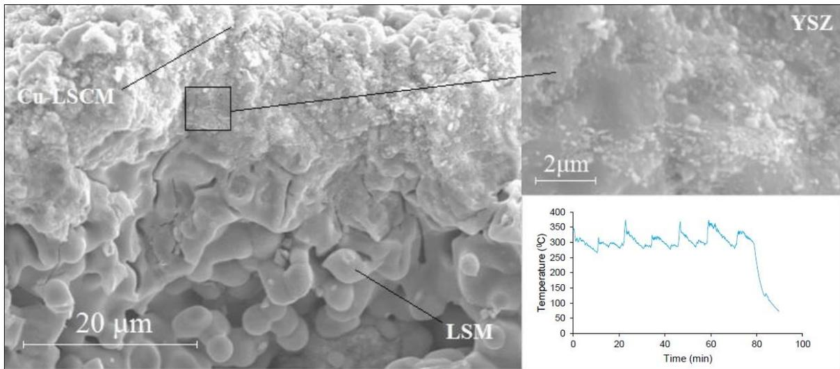
Fig 4. Cross section SEM of the composite Cu-LSCM/YSZ/LSM and substrate temperature profile of the Cu-LSCM deposition.
