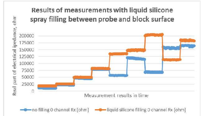
Fig.9 EIS measurements during the drying process of the reference block and block with liquid silicone spray filling between the probe and the measurement surface
