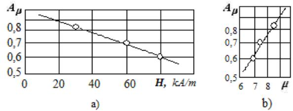
Fig. 2.  $A_\mu$  parameter data in (4) represented in semi-logarithmic (a) and logarithmic (b) coordinates to illustrate respective exponential and power dependencies of this parameter on the magnetising field intensity and magnetic permeability of the ‘matter’ of the quasi-solid filter-matrix.
