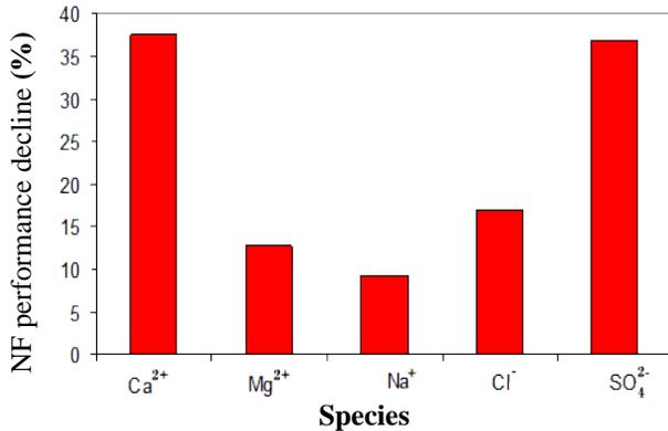
Fig 10. Percentage decline of the performance of NF during three years operation
