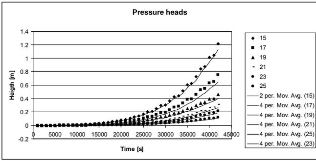
Fig. 8. Evolution of pressure head for different piezometer positions for dams with non permanent storage
