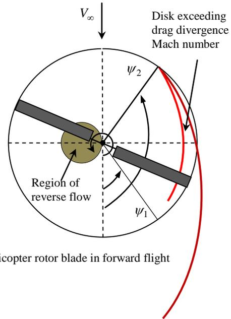
Fig. 1 helicopter rotor blade in forward flight
