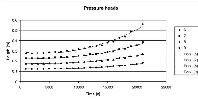
Fig. 4. Evolution of pressure head for different piezometer positions for dams with permanent storage
