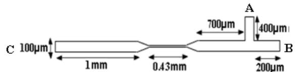
Figure 1. A typical convergence-divergence shape micro fluidic channel.
