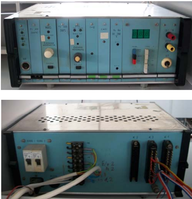
Fig. 2 A photo of the current converter/control unit – the front (a) and the back side (b)
