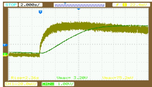
Fig. 6 the output sequencing with 47 \text{ k}\Omega load TEC12708
