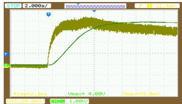
Fig. 7 the output with 47 \text{ k}\Omega load MCHPE-127-10-08-E
