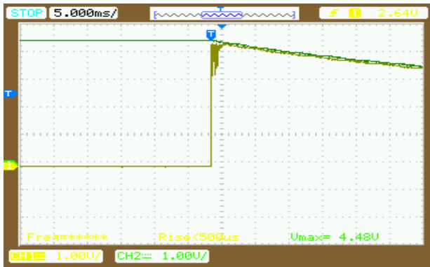
Fig. 4 the output of the device with TEC module MCHPE-127-10-08-E
