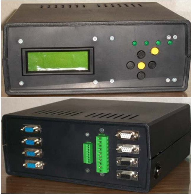
Fig. 5 A photo of the new designed converter/control unit – the front (a) and the back side (b)
