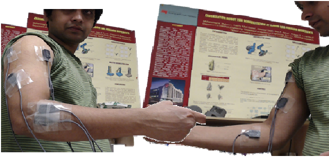
Fig. 8 Electrode placement for elbow joint flexion/extension, forearm pronation supination and shoulder joint vertical flexion/extension motion
