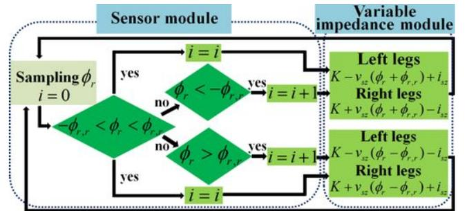
Fig. 13. Variable impedance control:  $\phi_{r,r}$  is reference roll angle.
