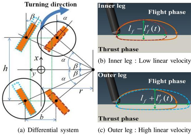
Fig. 5. Turning of robot : Differential system of 4WS
