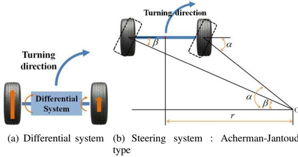
Fig. 2. Differential system and steering system in a car
