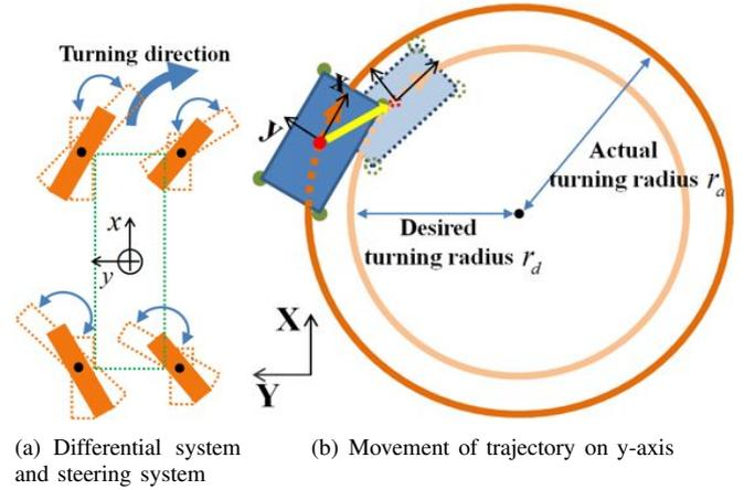
Fig. 16. Compensation of turning error
