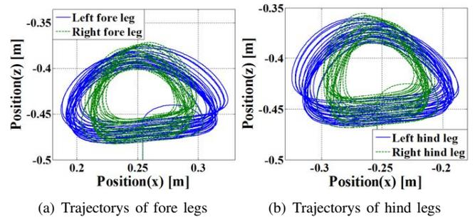
Fig. 21. Trace of foot trajectory
