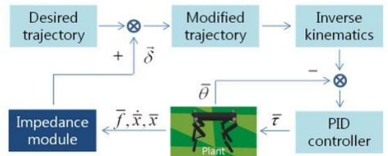
Fig. 8. Impedance control block diagram
