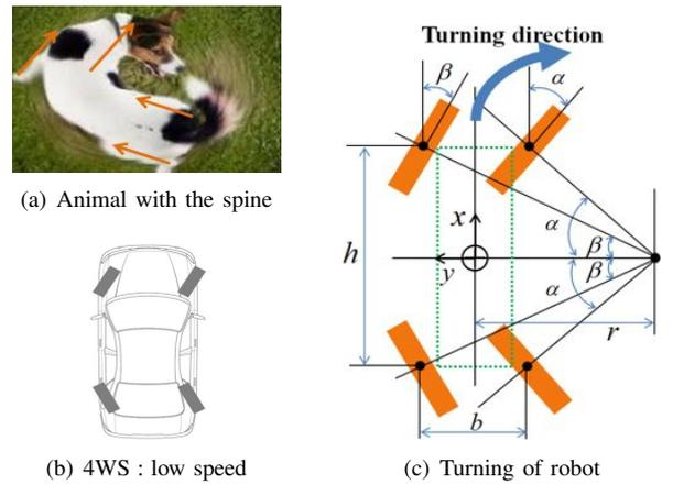
Fig. 4. Turning of robot : Differential system of 4WS
