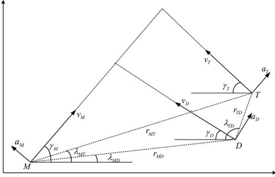
Fig. 1 Target-attacker-defender engagement geometry.
