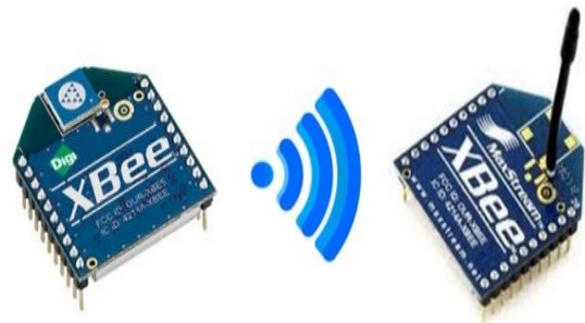
Figure 2.c: Transmission Module Xbee
