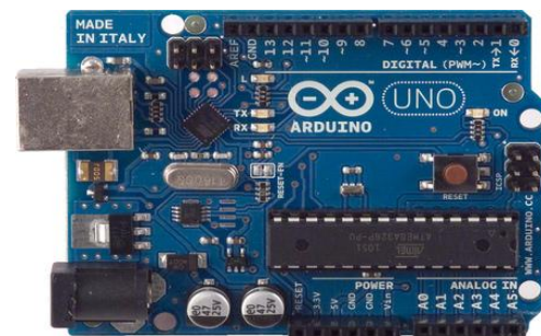
Figure 2.b: Arduino-uno system board
