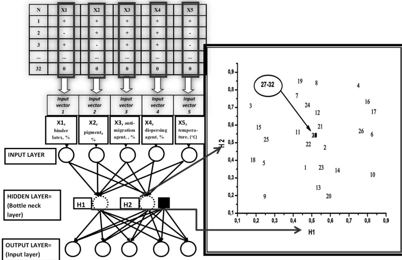
Fig. 3. The architecture of FFBN neural network applied in the study and projection of 32 objects (corresponding to the 32 experimental settings) from two hidden layers H1/H2 into 2D map.
