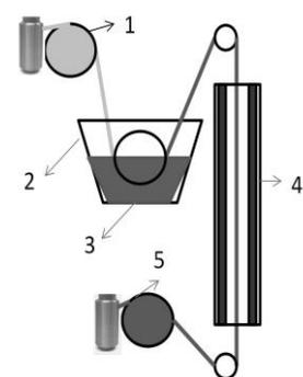
Fig. 1. The operation scheme of pigment dyeing module.
