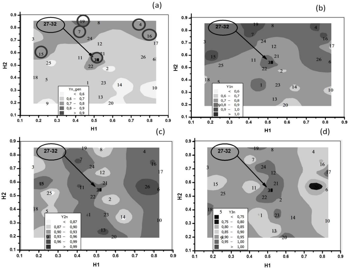
Fig. 4. The map of 32 factor settings (experimental condition) overlapped with contour plots of (a)-generalized response  $Y_{n\_gen}$  and individual responses: (b)-  $Y_{1n}$ - color strength, (c)-  $Y_{2n}$ - tensile strength and (d)-  $Y_{3n}$ - elongation to break.
