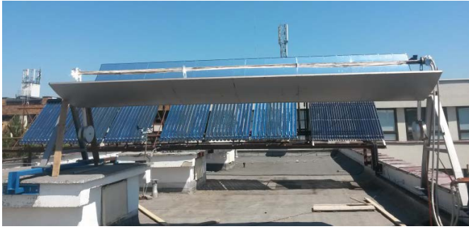
Fig. 6. Turning of the trough solar collector during the measurement
