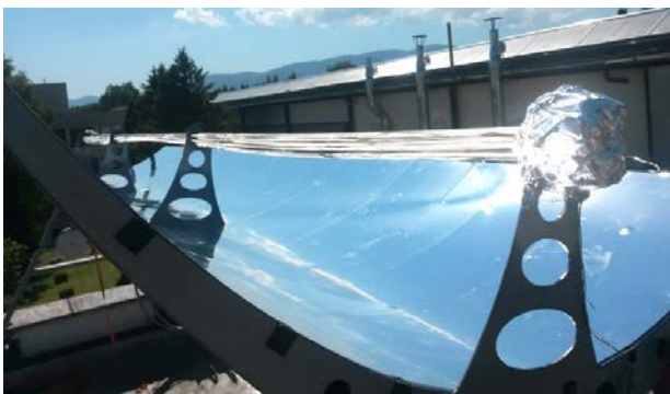
Fig. 7 Change the shape geometry of pipes in the focal heat exchanger.
