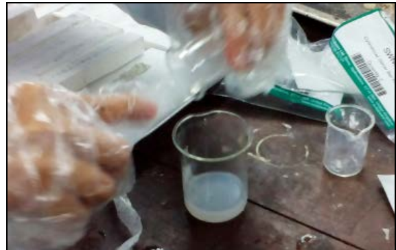
Fig. 3 Mix Silicone Ecoflex with its hardener
