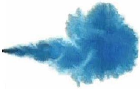
Fig. 6 The head of the starting jet in test TN1 is arrested by friction.
