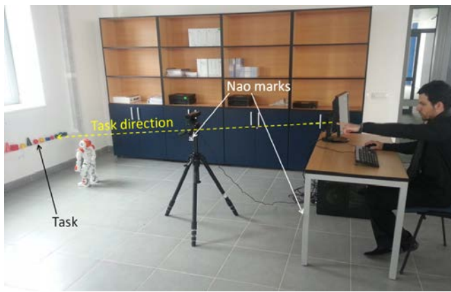
Fig. 8. The testing room. The user indicates the location by pointing and verbally the task to be executed
