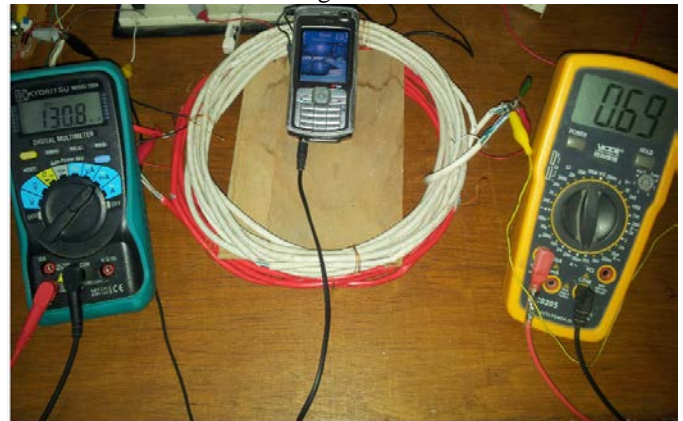
Fig.5 Wireless charging system for Nokia N70
