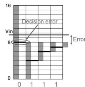
Fig. 2. Example of decision error due to incomplete DAC settling.
