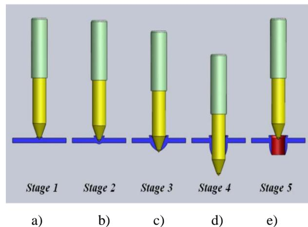
Fig.1. Stages of Friction Drilling.
