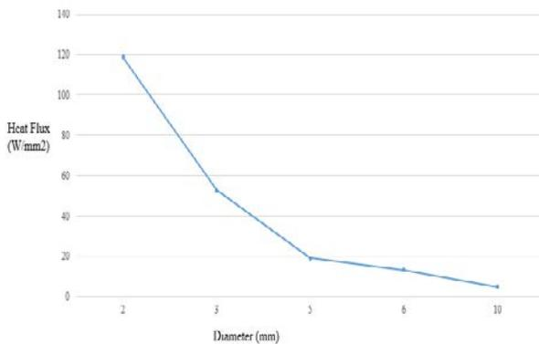
Fig 4 Effect of tool diameter on heat flux
