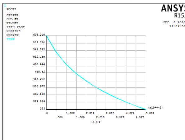
Fig. 8 Temperature vs. Distance (AA 6061 T6)
