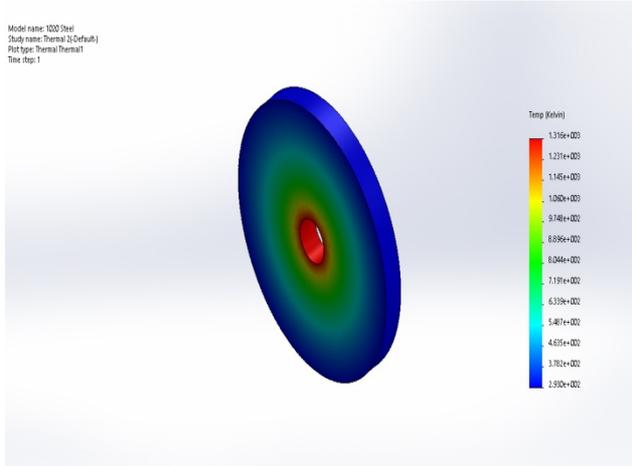
Fig. 5 Temperature Distribution in 1020 Steel during Friction Drilling
