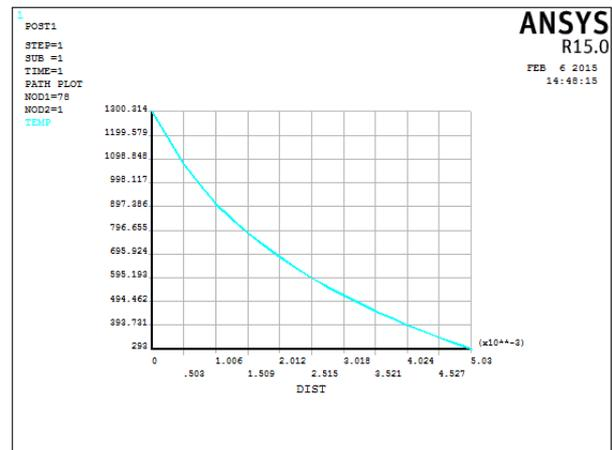
Fig. 6 Temperature vs. Distance (for 1020 Steel)
