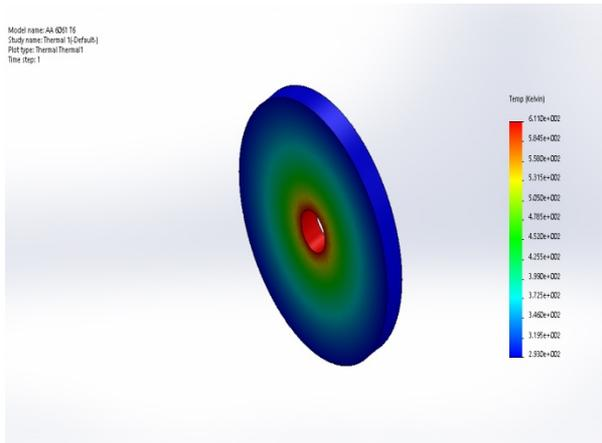
Fig. 7 Temperature Distribution in AA 6061 T6 during Friction Drilling
