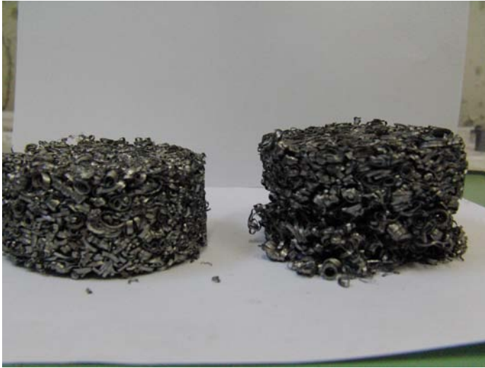
Fig.3. Briquettes from Armco iron chips with 80 mm diameter: left – after one impact; right – after two impacts
