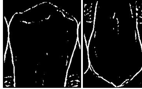
Figure 5: Point detector after applying median filter
