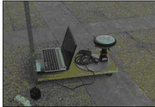
Fig. 6 simultaneous positioning Laser Scanner and GPS on "mobile equipped trolley"
