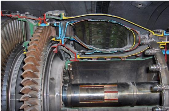
Fig. 1 Combustion chamber
