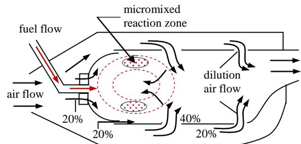
Fig. 2 Combustion chamber flow pattern
