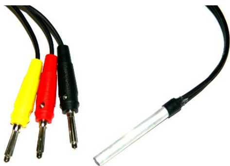
Fig. 5 Self-produces sensor with cables and case
