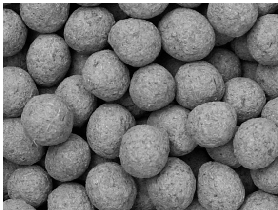
Fig. 2. spherical organometallic granules on the base of flax shive
