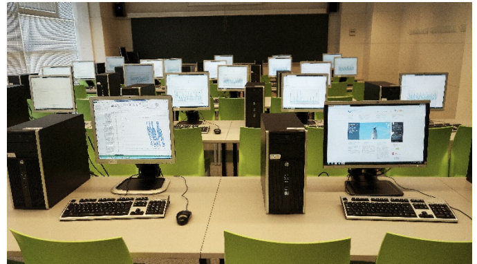
Fig. 7 Computer lab used to execute the simulations. Note that all the computers compose a farm that shares the model and executes a part of the experiment, uploading the results to a central server.
