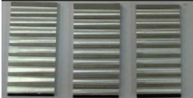
Fig. 2: Machined specimens of Al7075 alloy
