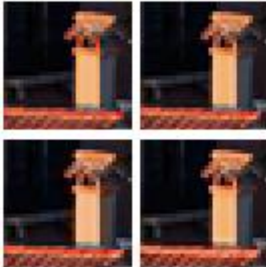
Fig. 4 Top left: original image; Top right: the 4:2:2 image subsampling; Bottom left: the 4:1:1 image subsampling; Bottom right: the 4:2:0 image subsampling
