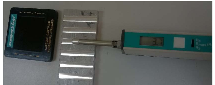
Fig. 5: Machined specimen and surface tester
