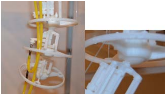
Fig. 7. Element of robotic arm, a-robot ansamble, b-spherical articulation detail
