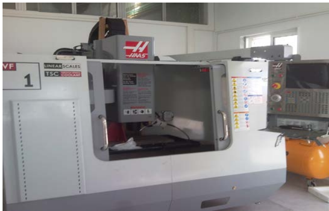
Fig. 3: HAAS VF1CNC machine centre (7500 rpm, 15 KW)
