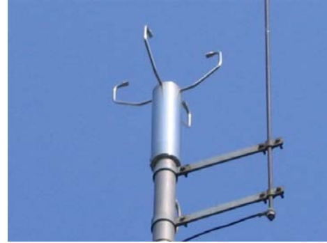
Fig. 2 Wind recording station VS425
