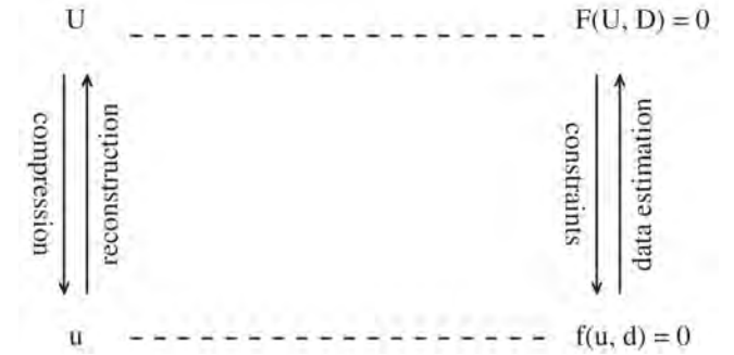
Fig. 1. Schematics of HMM general framework [16]. Two modelling scales are coupled by means of translation operators. The compression operator defines rules to refine the description and the reconstruction operator averages micro-scale data to feed the macro-scale.
