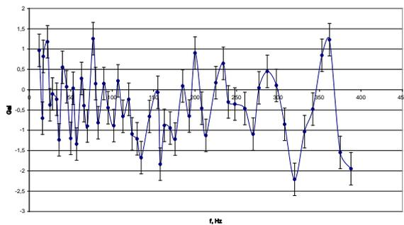
Fig.3. The frequency dependence of free falling acceleration of the container with horizontally positioned rotor; the changes of FFA ( $Gal$ ) relatively to the value of FFA with the stopped rotor have been shown.
